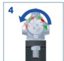
4 Coupling automatically locks on
